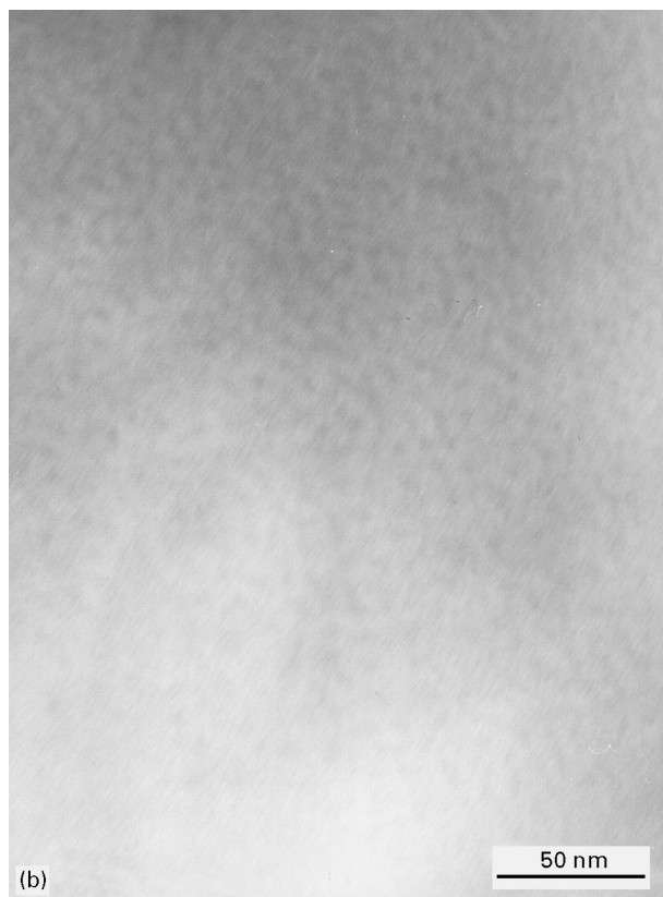
Figure 1 Bright field TEM micrographs of as-cast glass at (a) low magnification and (b) high magnification.
